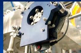
The speed at which the stoppers are placed is synchronized with the machine's outlet (up to 4000 BPH)
